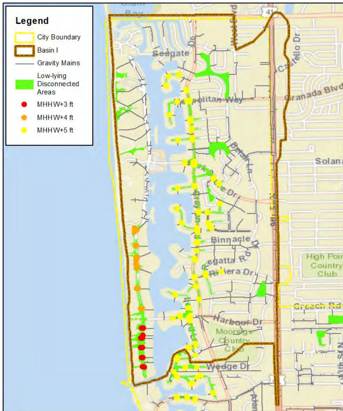
Figure 8-9 Exposure of Inlets to Backflow Flooding and Groundwater Effects in Basin 1
