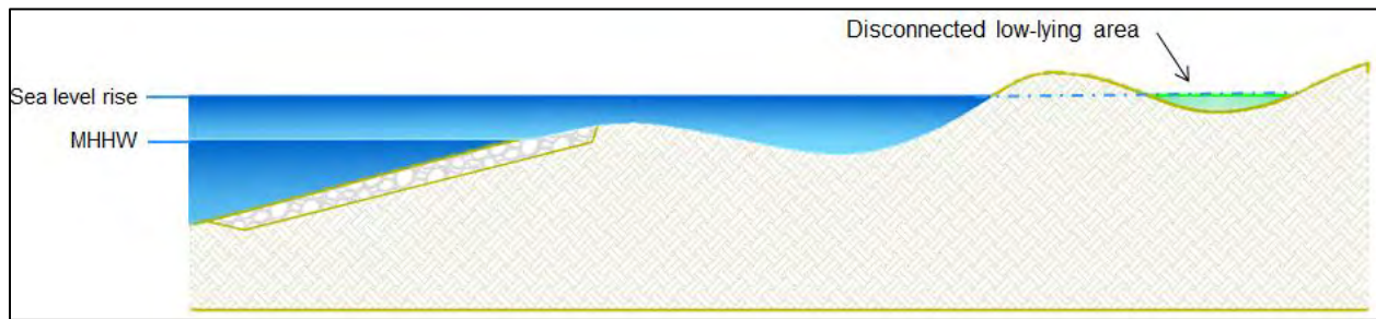
Figure 8-4 Example Shoreline Cross Section Showing Disconnected Low-Lying Area
